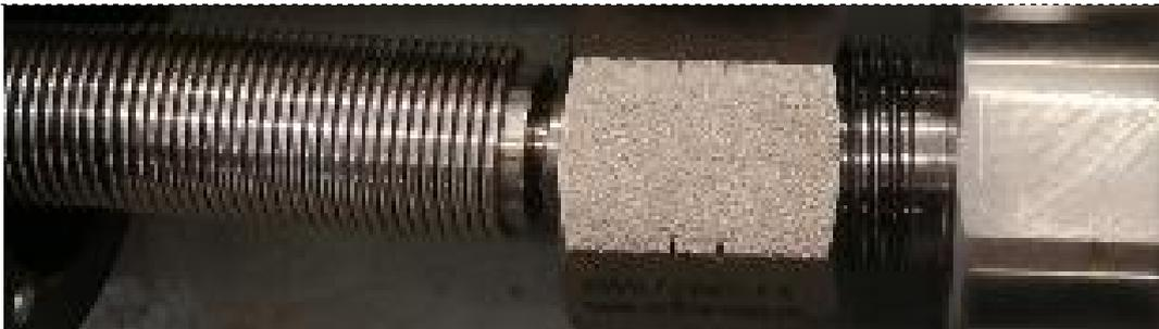
Connect and fasten the hydrogen refueling hose and hydrogen refueling nozzle
